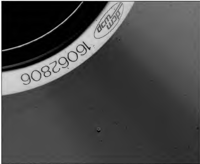
Fig. 9.1. Disc with an intentionally damaged sector (a small "volcano" a little below the middle of the screen). Using specialized equipment allows you to burn the surface exactly in the center of the spiral track
